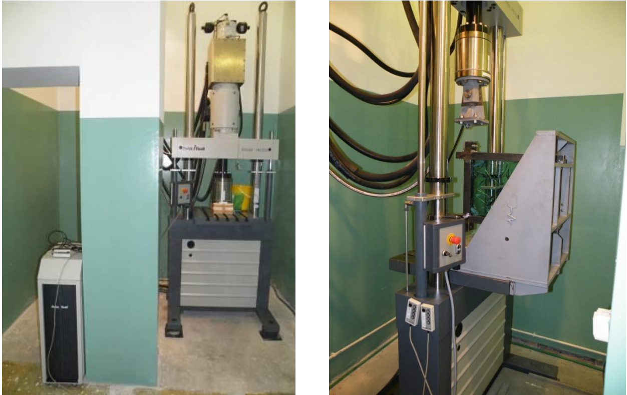
Figure 6. Servo hydraulic machine for dynamic and static testing ZWICK Roell HB - 250
